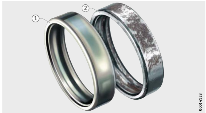
Figure 7 Bearing rings after the salt spray test
