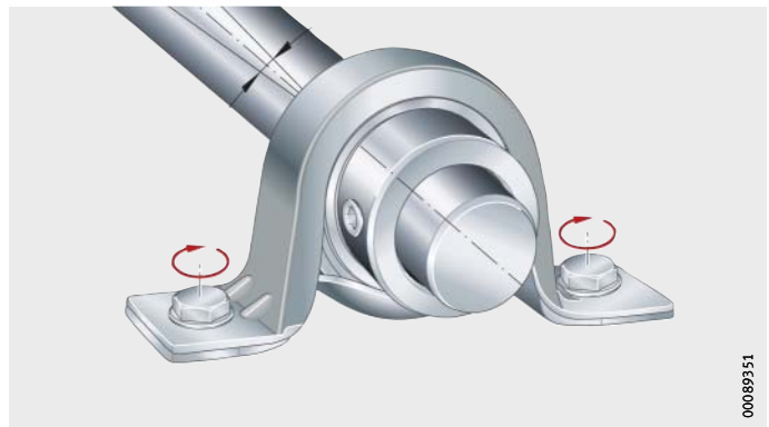
Figure 12 Screw mounting the housing finger tight
