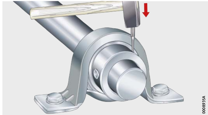
Figure 13 Tensioning the eccentric locking collar
