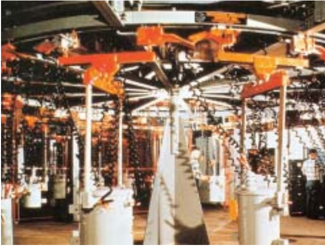
Power-and-free conveyor system
