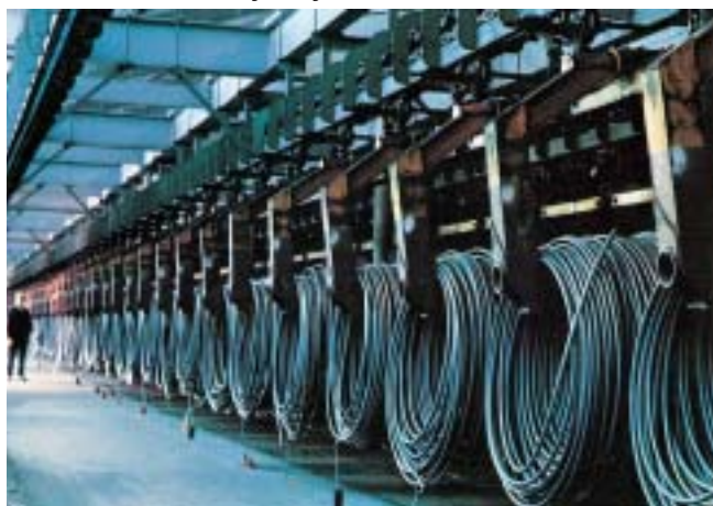
Power & free conveyor system
